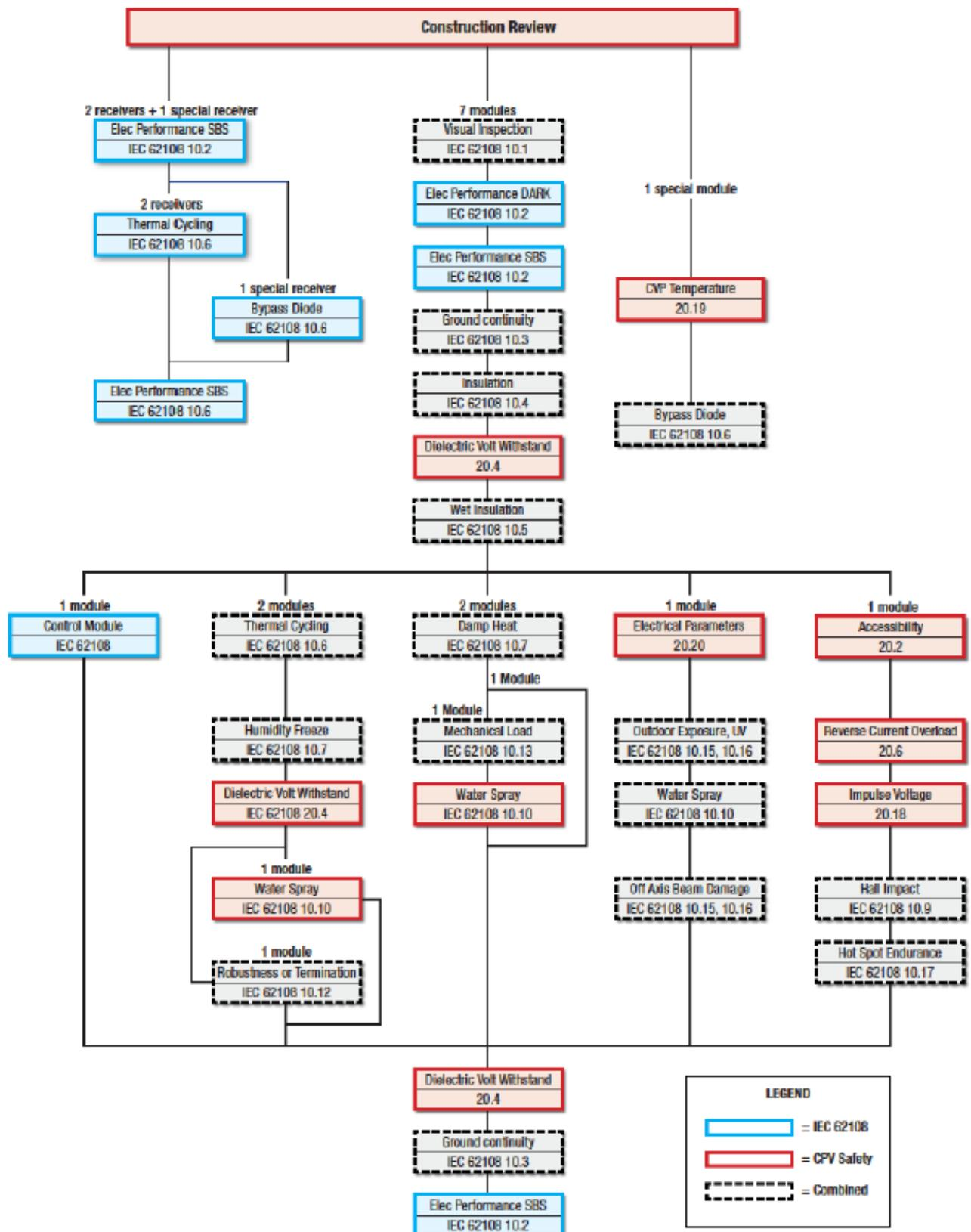
**Annex 1.4: Tests sequences for X1/X3, X2 and X4 BIPV product (task 4.1)**
