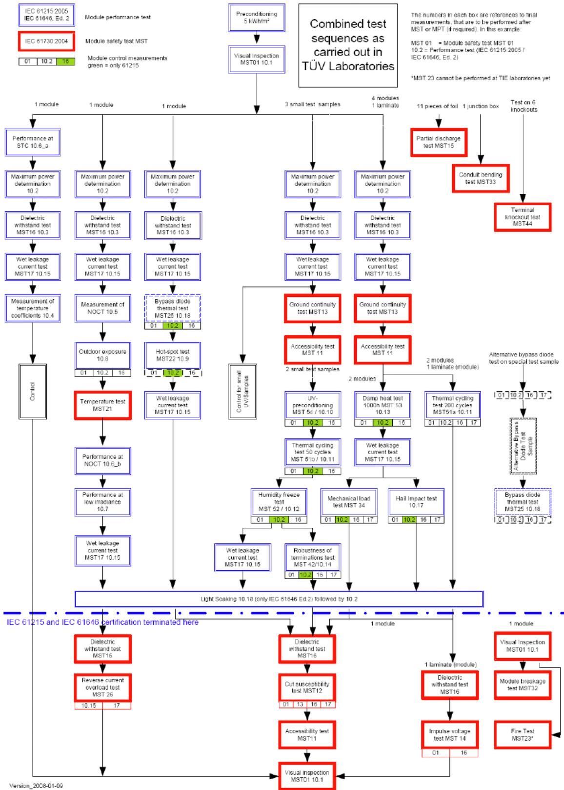
**Annex 1.3: Tests sequences for CPV modules**
