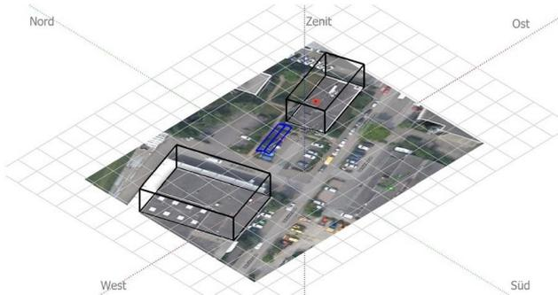
Location preferred by Flisom, close to the street with less shadowing and 7.3 MWh/year estimated production.
