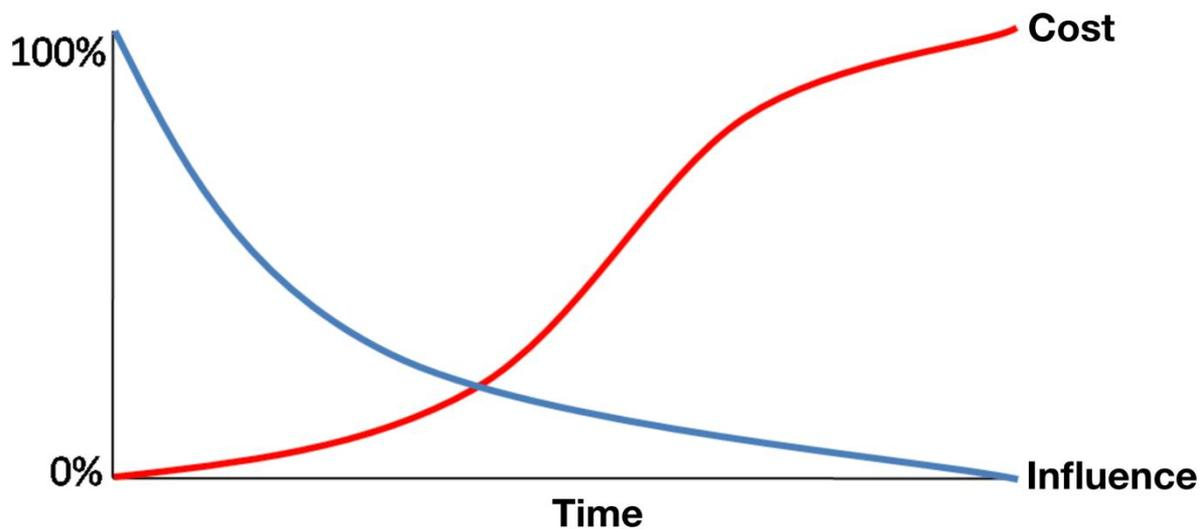
**Figure 2.1** The graph shows how the cost of design changes are increasing during the design process while the influence on the design becomes less.
